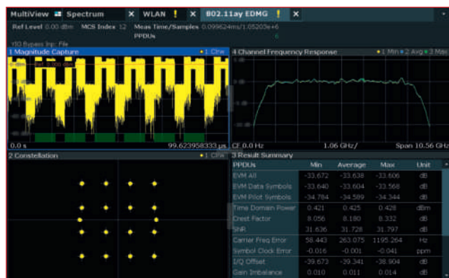
▲ Fig. 2 IEEE802.11ay channel bonded signal spanning 8 GHz.
