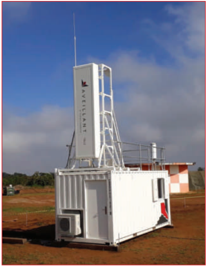
▲ Fig. 4 Radar developed for long-range detection, tracking and recognition of drones.
